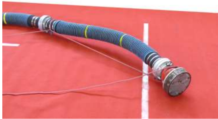
Fig. 13: Placing the suction head beyond the red lath
