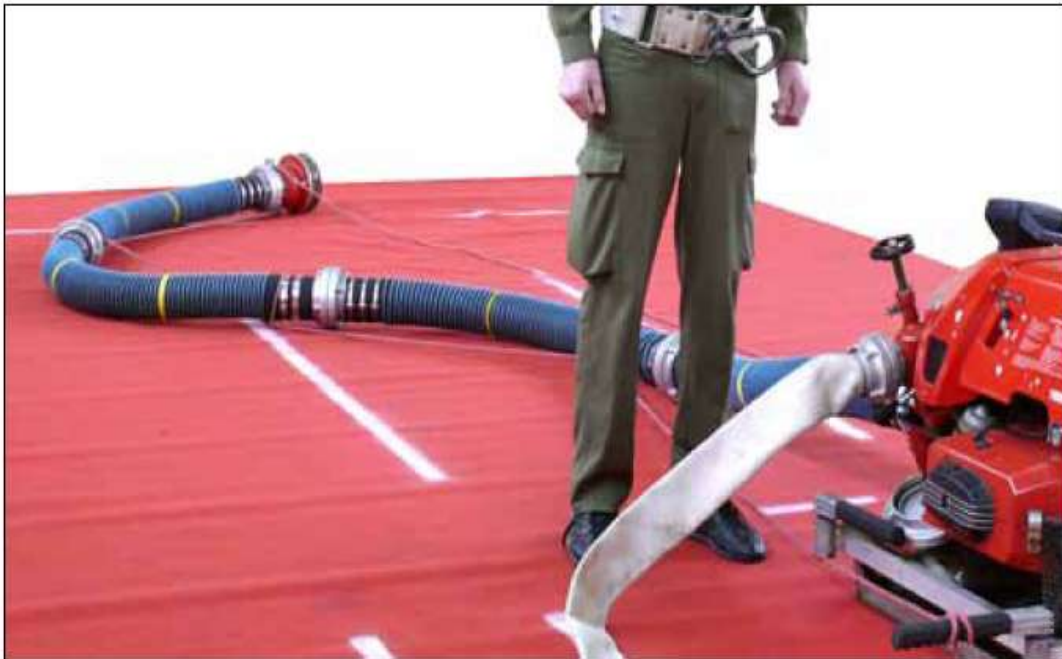
Fig. 16: Attaching the suction hose rope to the portable pump
