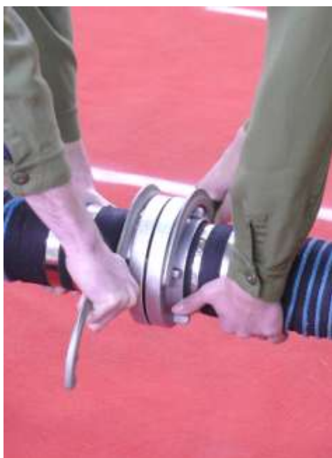
Fig.8b: Putting on the coupling keys and coupling the suction hoses
