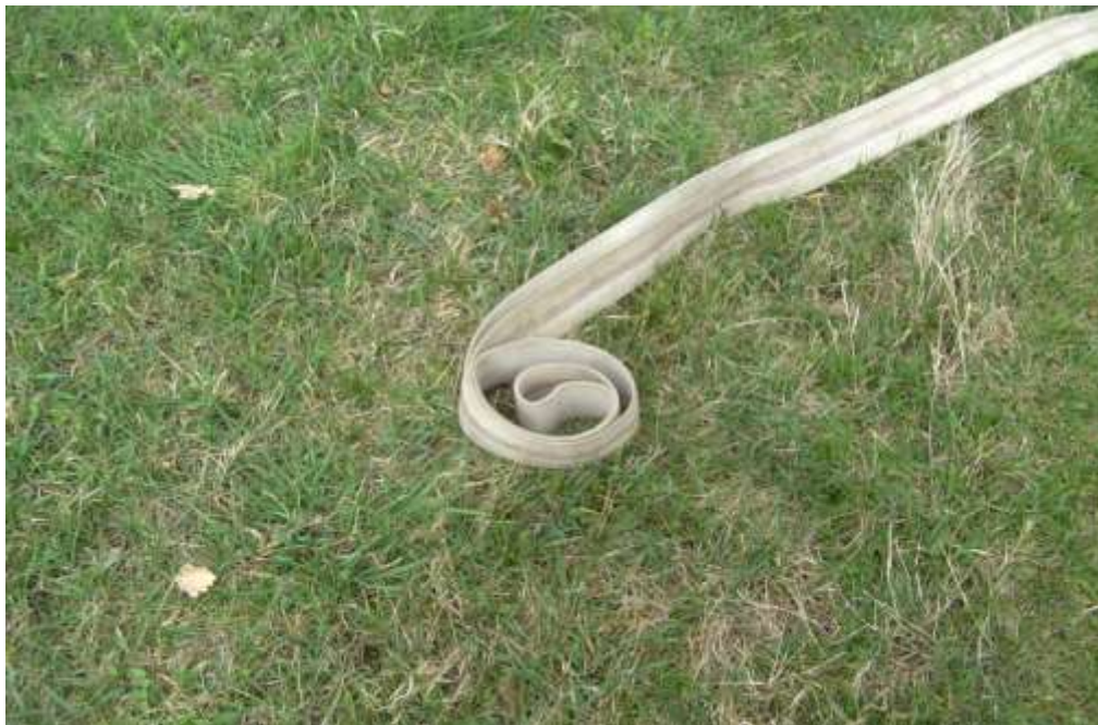
Fig. 21b Badly laid-out pressure hose „snail“
