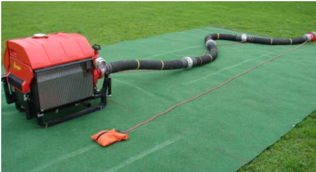
Fig. 15.: Position of the rope bag with the valve rope
